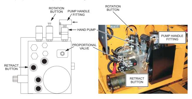
Figure 3-5. Hand Pump and Controls for Manual Lift Operation
